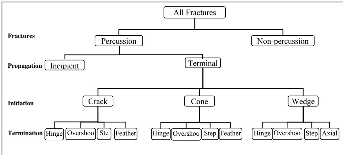
**Figure F1** Classification scheme for percussion fractures (Cotterell and Kamminga, 1987).
